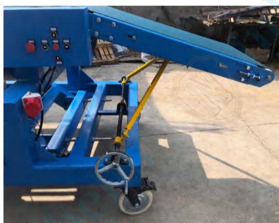
End slave section height is adjustable by hand wheel
