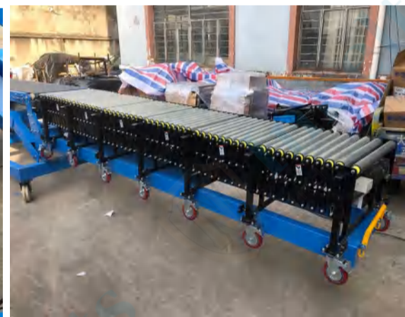
7.2m flexible powered roller conveyor
