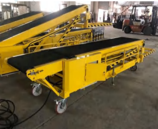
The front tongue conveyor can be removed when not use
