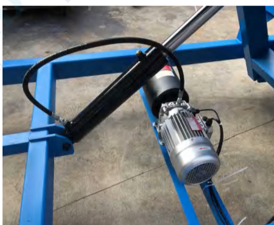
With hydraulic power unit for height adjustment
