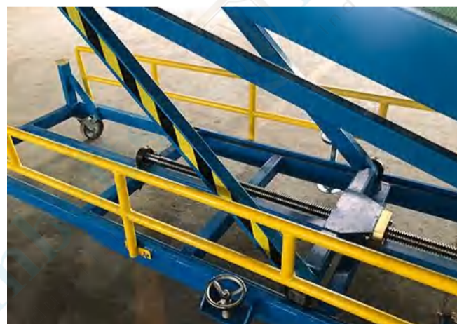
Side safety guide to prevent people down into the machine
