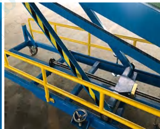
Safety guard to prevent people down into the machine
