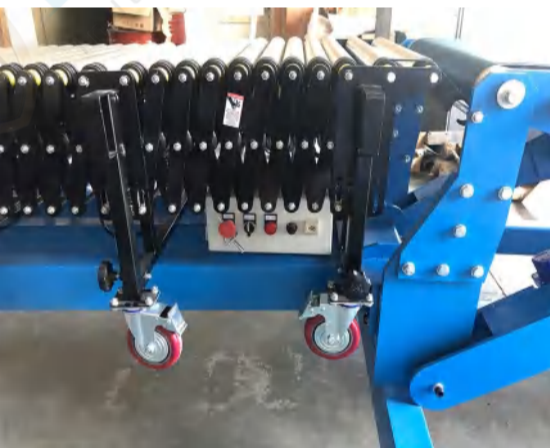
Flexible conveyor with independent control box
