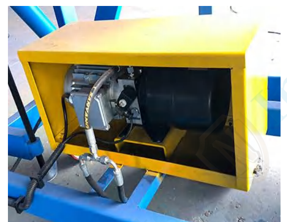
Hydraulic power unit
