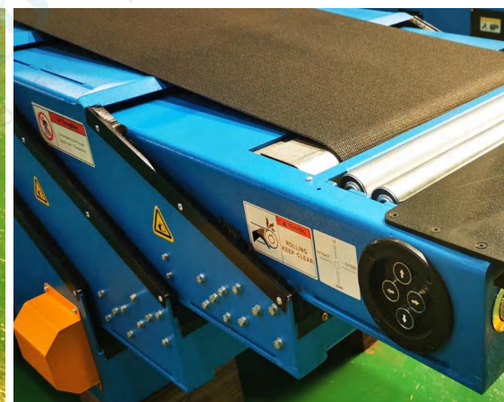
Control extend and retract on both side of the conveyor
