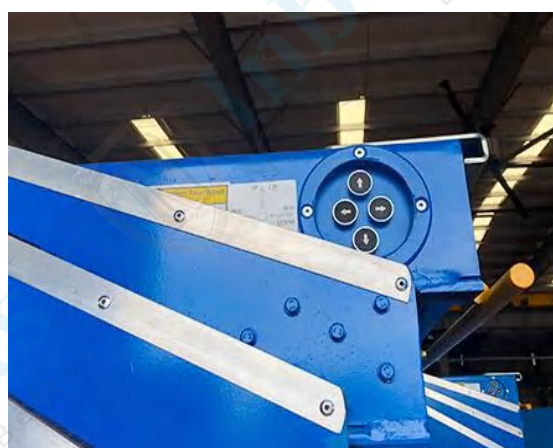
Side control panel to extend and retract the conveyor
