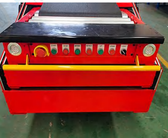
Front head control panel
