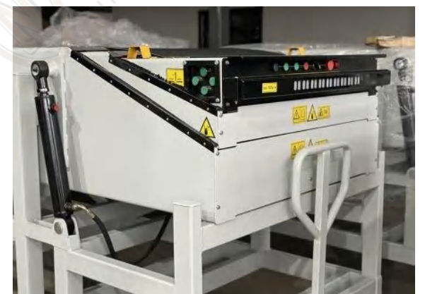
Front control panel for adjust length and height, control loading and unloading direction
