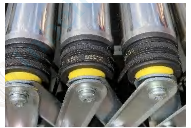
High Quality V Belt for Roller Driving
