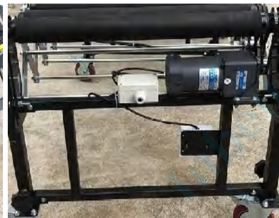
Each pair of legs are reinforced by cross bar.
