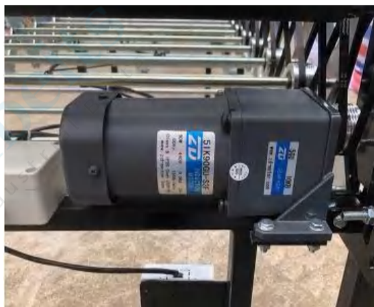
Every meter with one 90W/120W min motor
