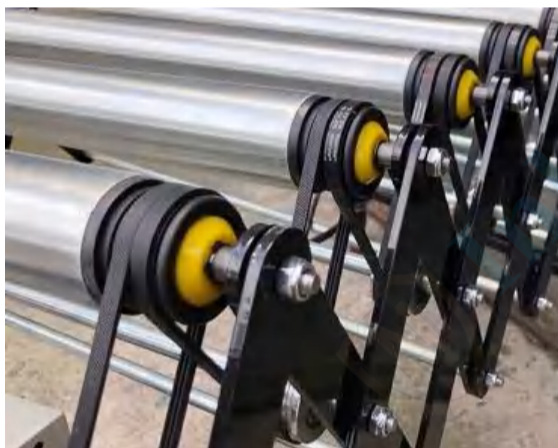
Rollers are driven by V belt
