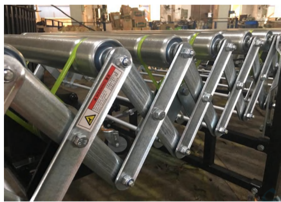
3.5mm thickness galvanized curved side links plate
