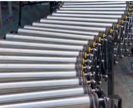
Dia 50mm galvanized steel rollers
