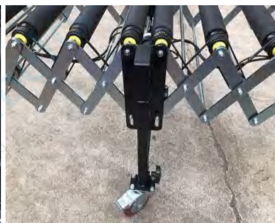
The legs and side links are connect by bolts.
