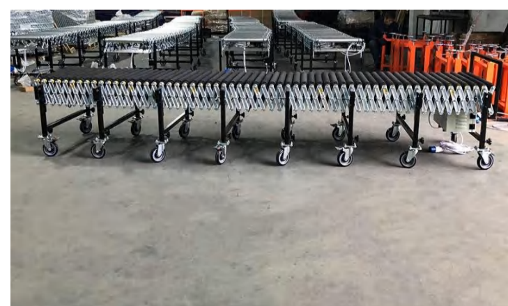
Mobile on 5" lockable swivel castors.
