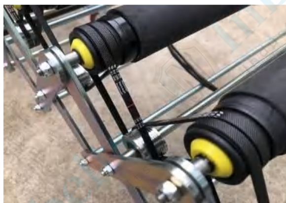
The rollers are driven by V belt
