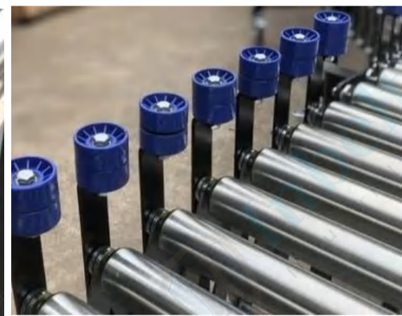
Guide wheels to keep goods from falling off
