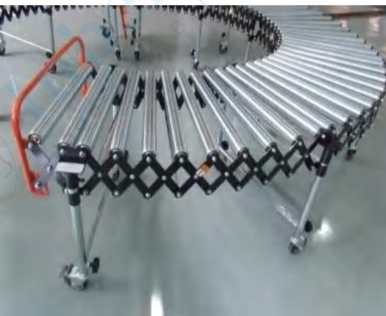
50*1.5mm galvanized steel roller
