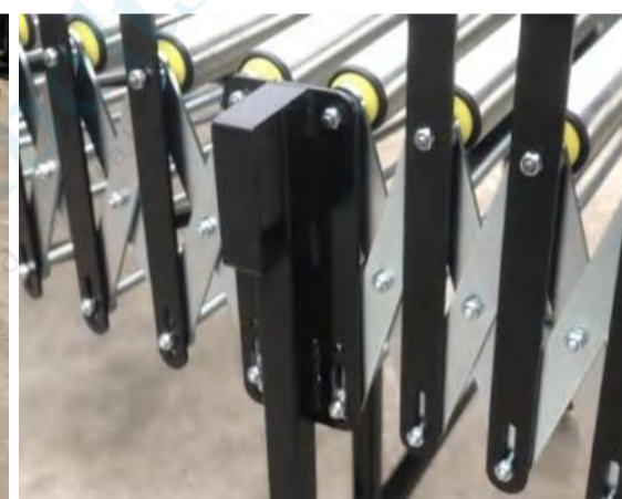
Legs with handle for movement
