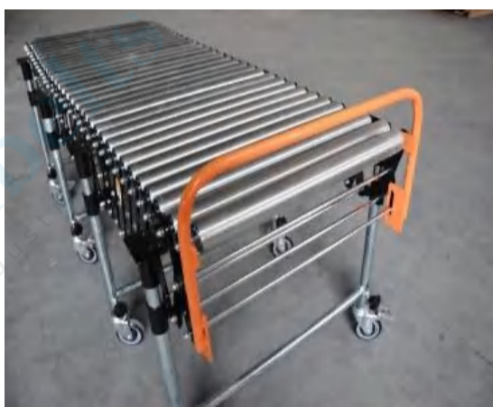
With end package stop bar
